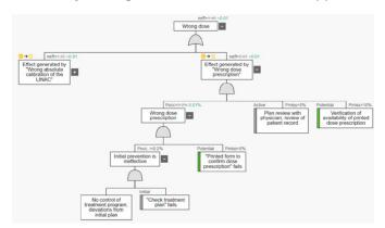
Figure 2. Example of fault tree for SGRT Breast Breath-Hold with top event "wrong dose" [8].
